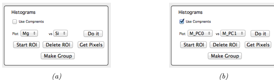
Figure 11: Histograms can be generated from either elemental- (left) or principle component maps (right). If the checkbox Use Components is active, the popup menus give access to principle component instead of element maps.
